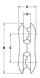
Pulling Rope Connectors are cast from high grade steel and all castings are 100% pull tested to ensure high quality. Pulling line connectors should be sized in accorance with the rated working load of the rope being used. These high strength connectors are shaped to pass around bullwheels under load.
