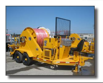
The DPT-40B is a proven hydrostatic pulling and tensioning system with hydraulic oil cooler and water cooled diesel engine. The DPT-40B is mounted on a dual axle trailer with leaf spring suspension with a reel capacity of 1828 mm (72") diameter, 1422 mm (56") wide and 2722 kg (6,000 lbs.).
